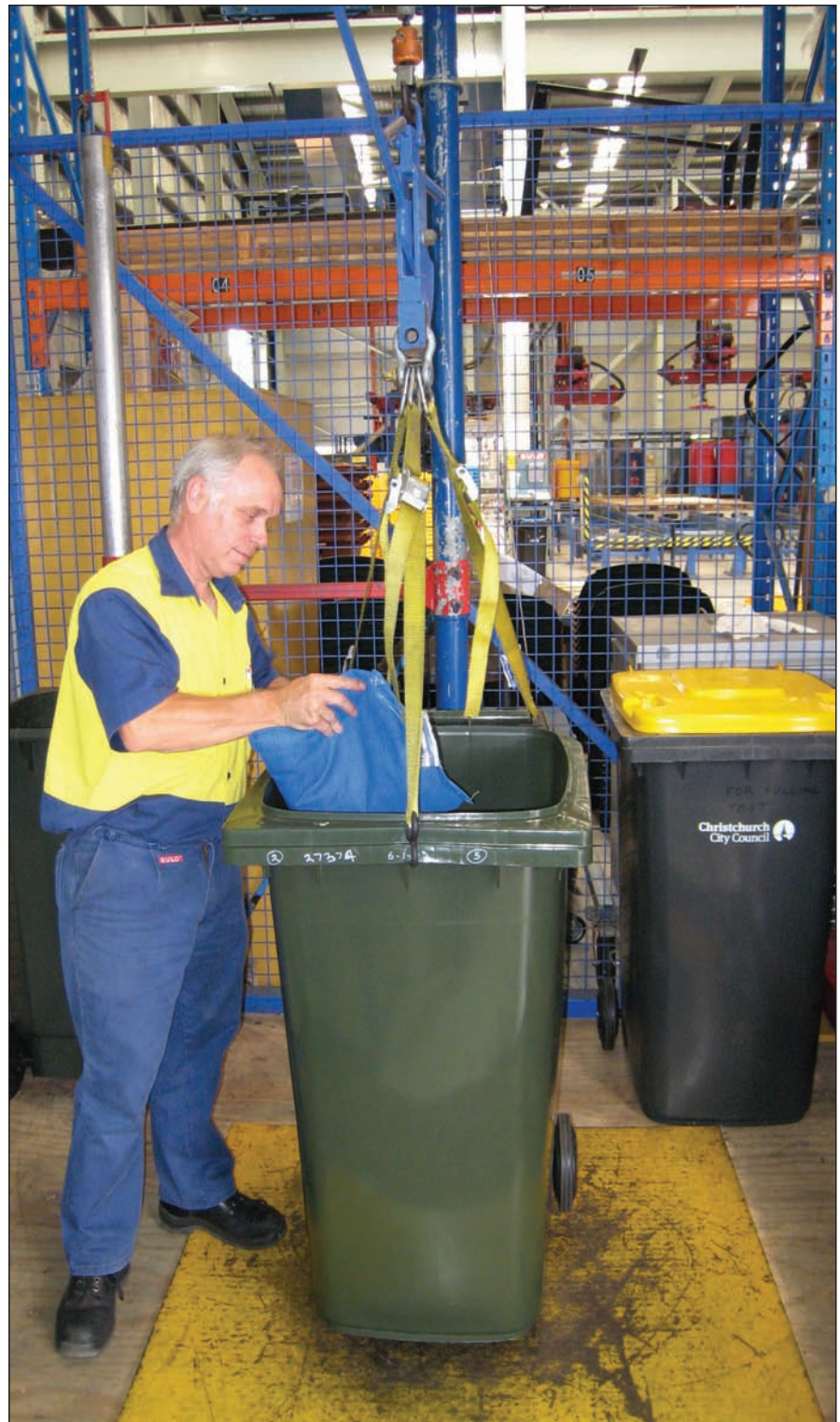
SULO's Quality Control Technician, Paul Render prepares an MGB for a drop test.
